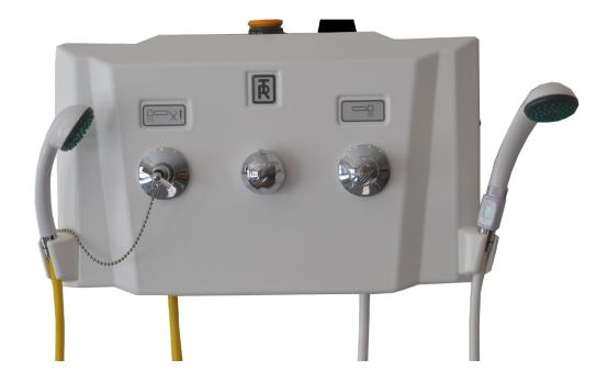
TR 2810 is a shower panel with a built in thermostatic mixing valve and separate on/off valves for the shower system and the cleaning system. The cleaning system runs on cold water to minimize inhalation when cleaning equipment, the panel has a built in bottle for cleaning detergent.
