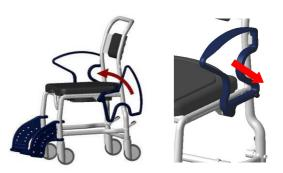
**4.** The back wheels are always locked for delivery. Lift up the locking levers to release the wheels.
